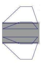
The fins are trapezoidal fin set. 4 fins are used for better stability tilted at an angle of 22.5. The fins are made of Carbon Fiber.
