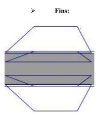
The fins are trapezoidal fin set. 4 fins are used for better stability tilted at an angle of 22.5. The fins are made of Carbon Fiber.
